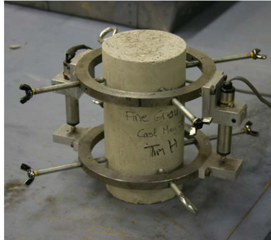
Figure 1: Compression Test Apparatus for Determining Strain
