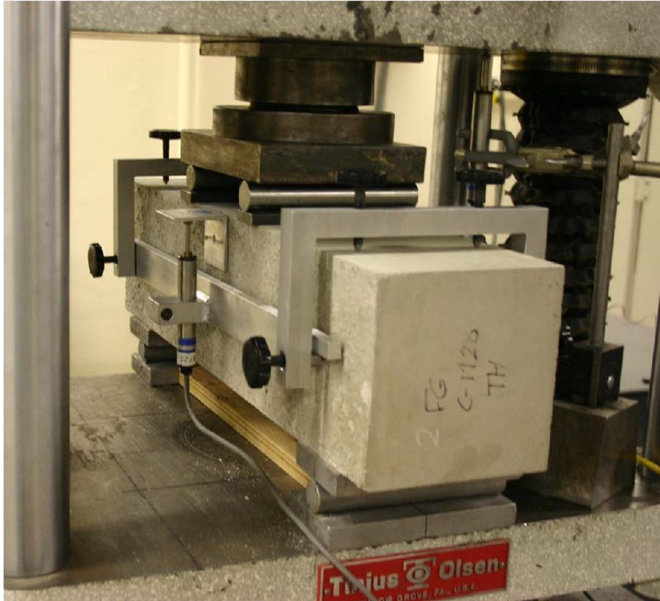
Figure 2: Flexural Test Setup
