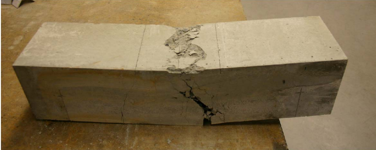
Figure 8: Ideal Failure, CG60 Specimen 1
