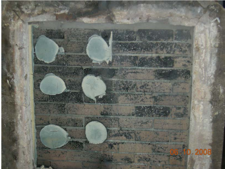
Figure 7: Exposed face at end of fire test
