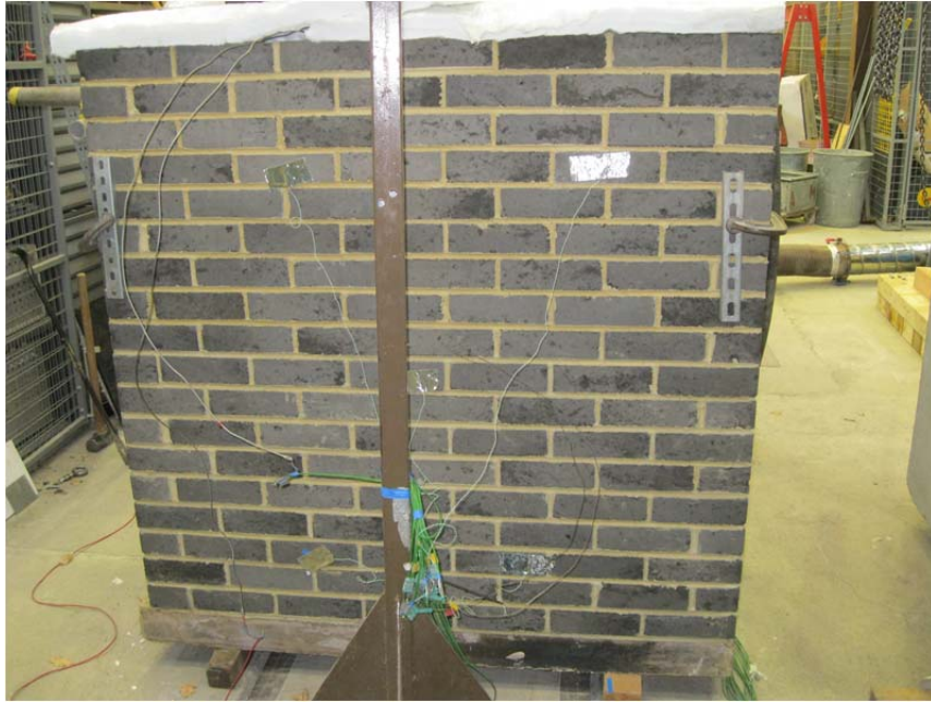
Figure 5: Unexposed face of masonry panel before start of fire test
