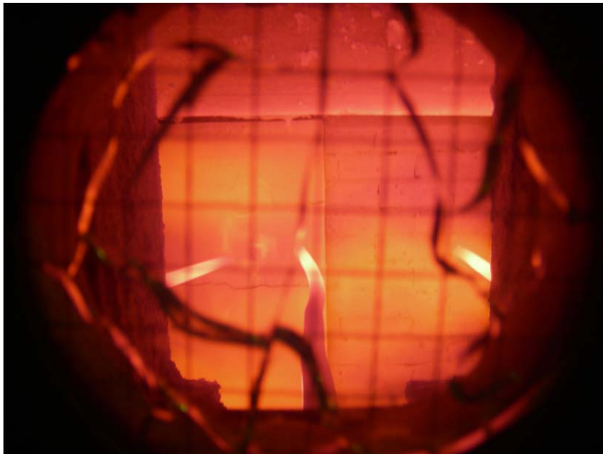
Figure 6: Exposed face – with and without plasterboard (note cracks in plasterboard)
