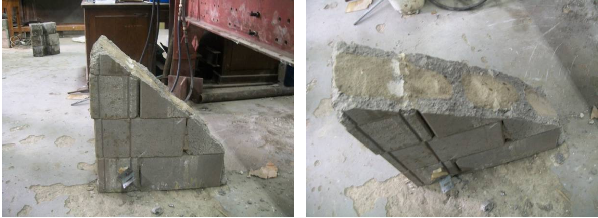
Figure 17: Failure Modes for Diagonal Tension (Shear) Test
