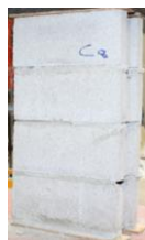
(a) Compression test on URM masonry
