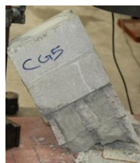
(b) Compression test on Grouted masonry
