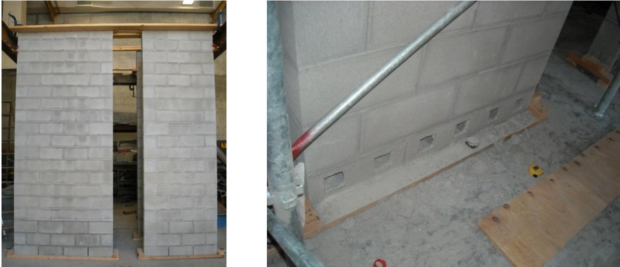
**Figure 7: (a) Wall Elevation and (b) Location of Cleanouts at Bottom of Wall**
