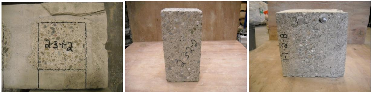
**Figure 11: (a), (b), Side of Compression Specimen and (c) Consolidation Specimen with Steel Reinforcement**
