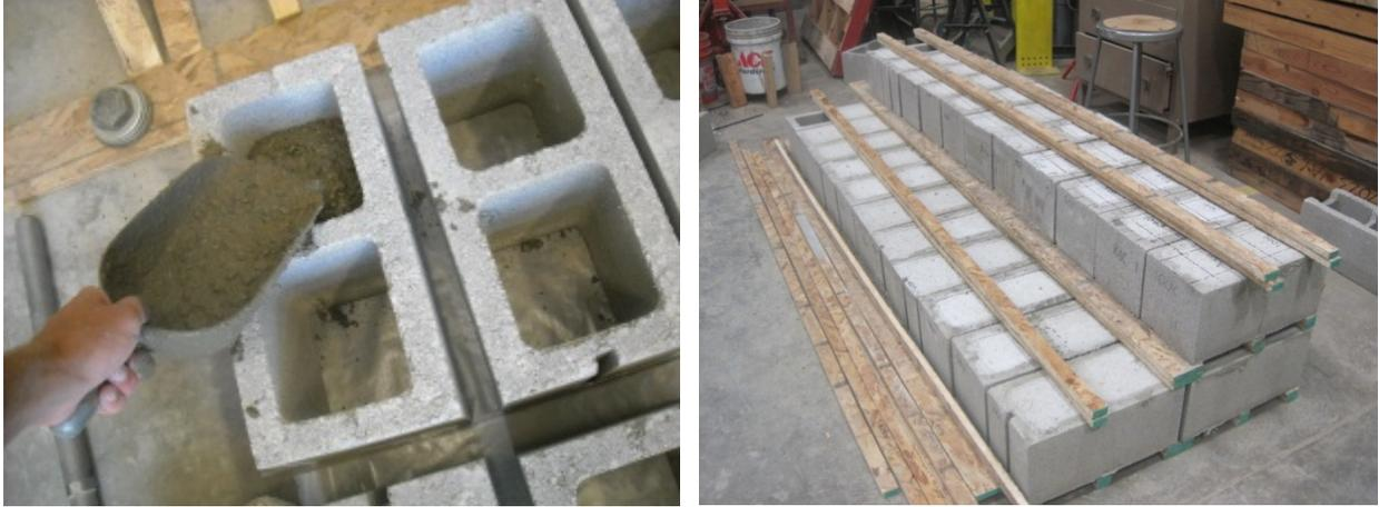
**Figure 3: (a) Placing Grout into Cores of CMUs and (b) Dry Curing Grout Specimens**
