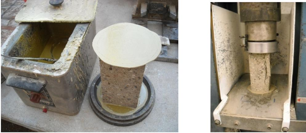
**Figure 5: (a) Capping of Grout Compression Specimens and (b) Compression Testing**
