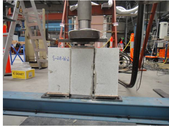
(b) Triplet failure (bond failure)
