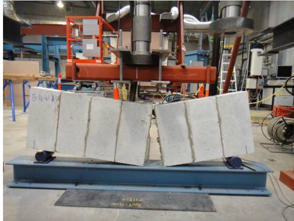
(a) Beam failure (bond failure)
