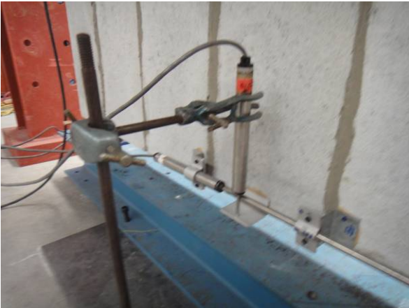
(a) LVDT positions on beam
