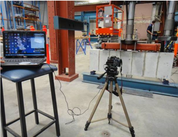
(c) Image acquiring of beam test
