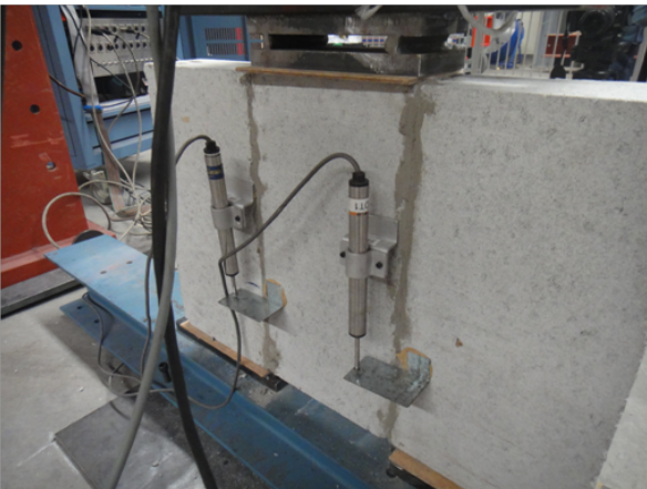
(b) LVDT positions on triplet
