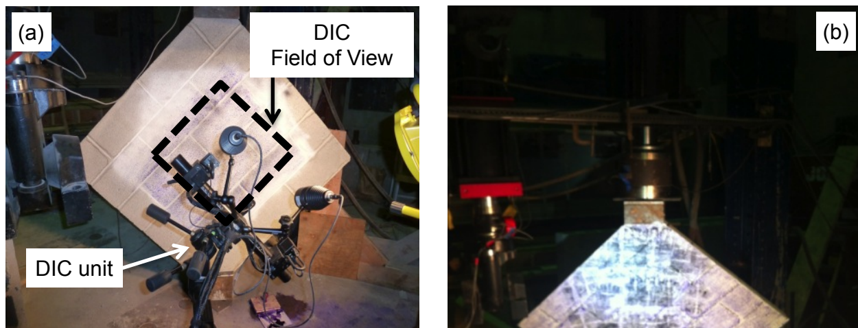
Figure 3: Diagonal compression tests: a) Hollow specimen and b) Grouted Specimen.
