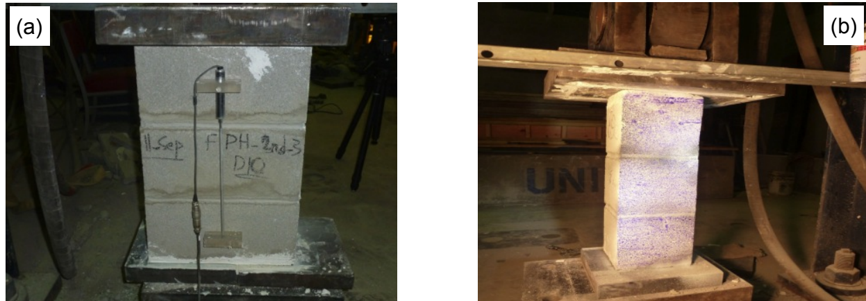
Figure 1: Axial compression tests of block prisms: a) Hollow specimen b) Half grouted specimen.
