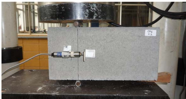
a) Concrete units in splitting tensile strength test.
