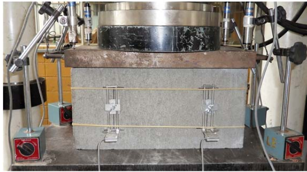
a) Concrete units in compressive strength test
