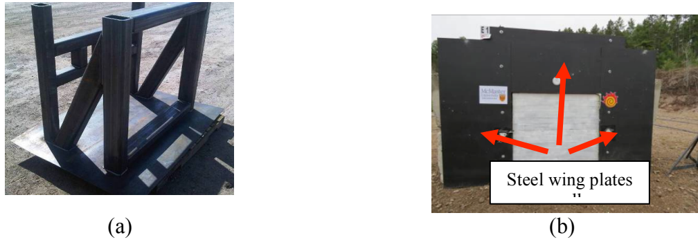
Fig. 4: Testing frame (a) main skeleton, and (b) final shape after installing wing walls
