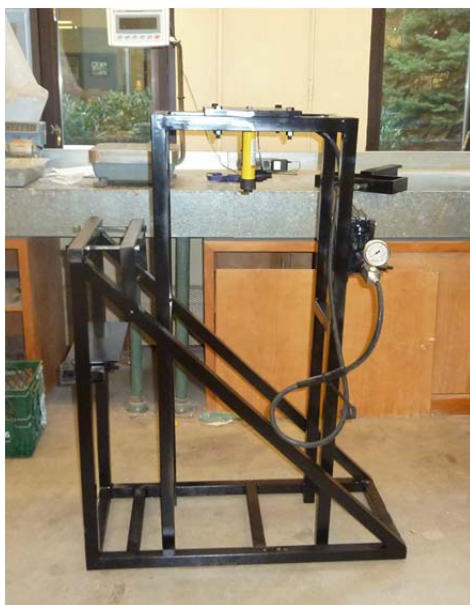
Figure 1: The Bond Wrench Was Constructed by the Gonzaga University Machine Shop in Accordance with ASTM C1072.
