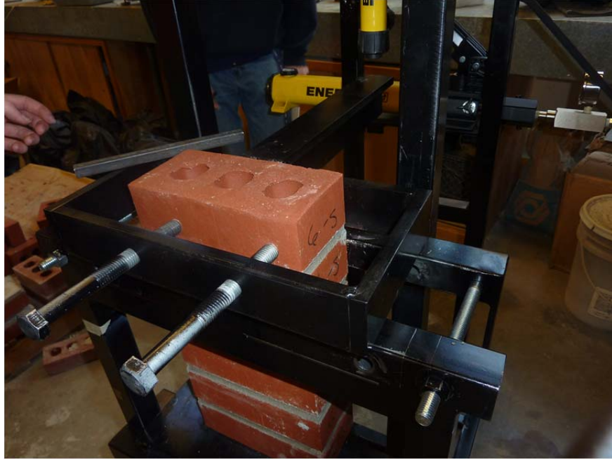
Figure 3: Prism Inserted in the Bond Wrench Prior to Testing.
