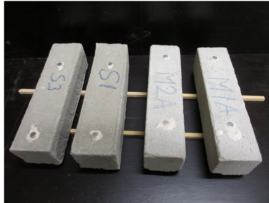
Figure 3: Masonry mortar prisms on wooden strips
