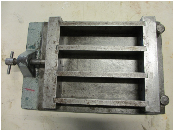
Figure 2: Steel and brick mould
