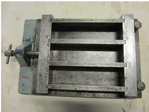
Figure 8: Steel mould and Calcium silicate mould
