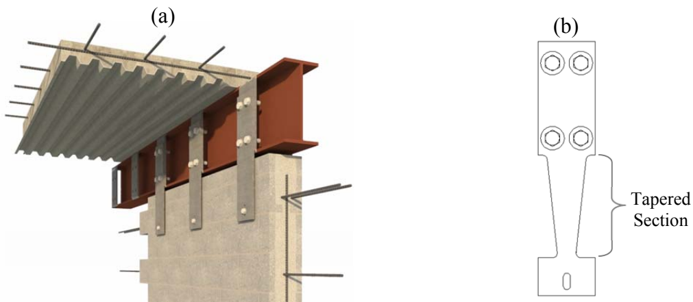
Figure 1: Type I Hybrid Detail (a) Link Plate Connectors from IMI (b) Fuse Connector
