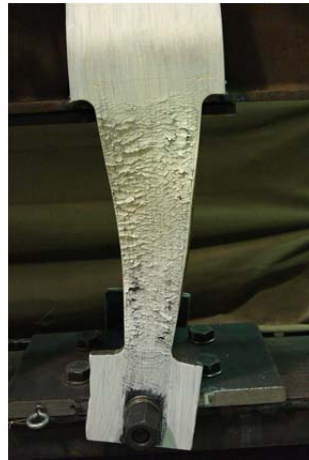
Figure 6 - Fuse plate connector with ductile flexing
