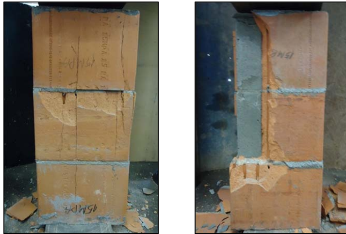
Figure 5: Characteristic rupture of the: (a) hollow prisms; (b) grouted prisms
