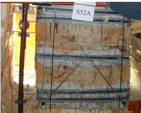
Figure 11: Failure by diagonal cracking and crushing of comp. toe
