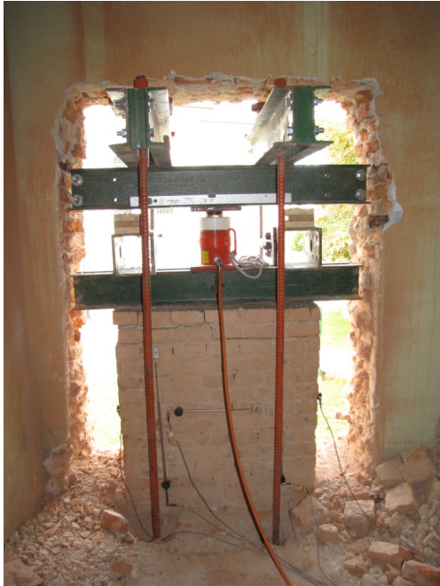
Figure 3: Compression test set up
