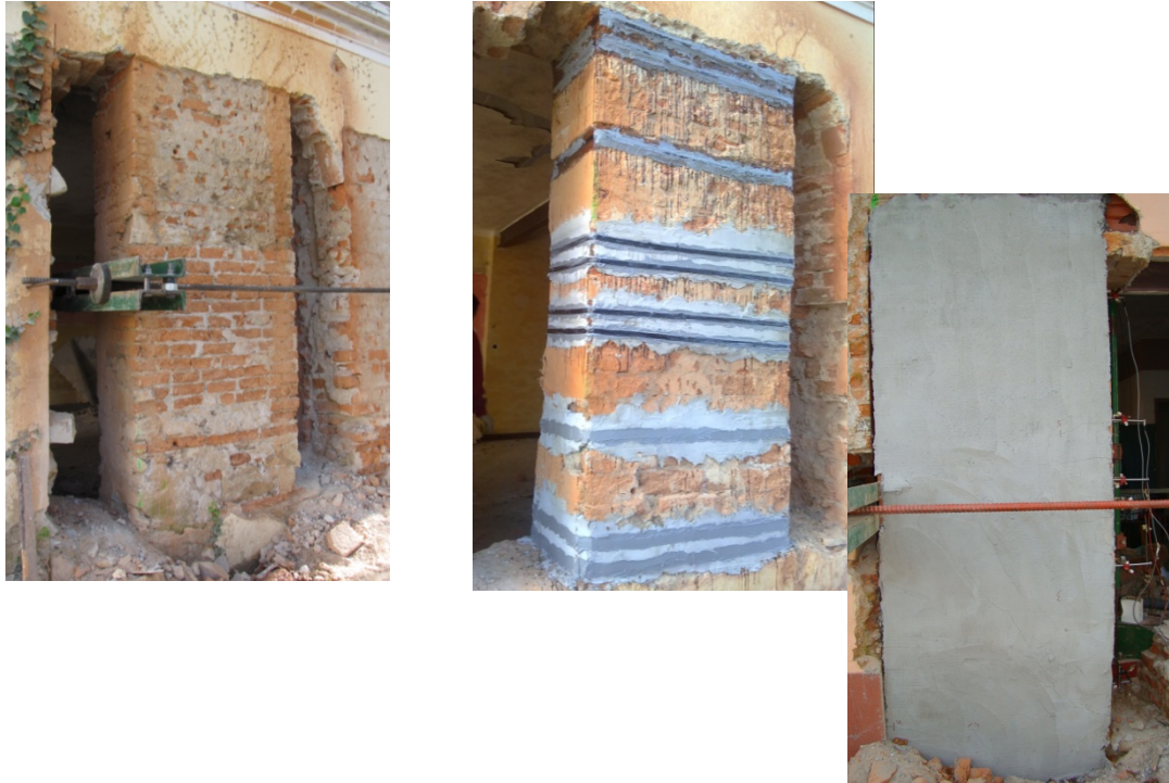
Figure 2 (a, b, c): Three configurations (un-strengthened R, with horizontal stripes S and mesh M) were prepared for shear testing
