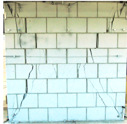
Figure 6: Hysteretic Response of Wall P3
