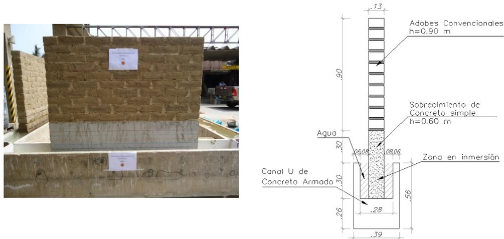
Figure 5: Concrete Plinth Wall – CW1
