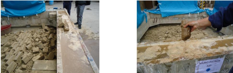
Figure 9: Overturned wall TW1 and condition of the adobes in the base.
