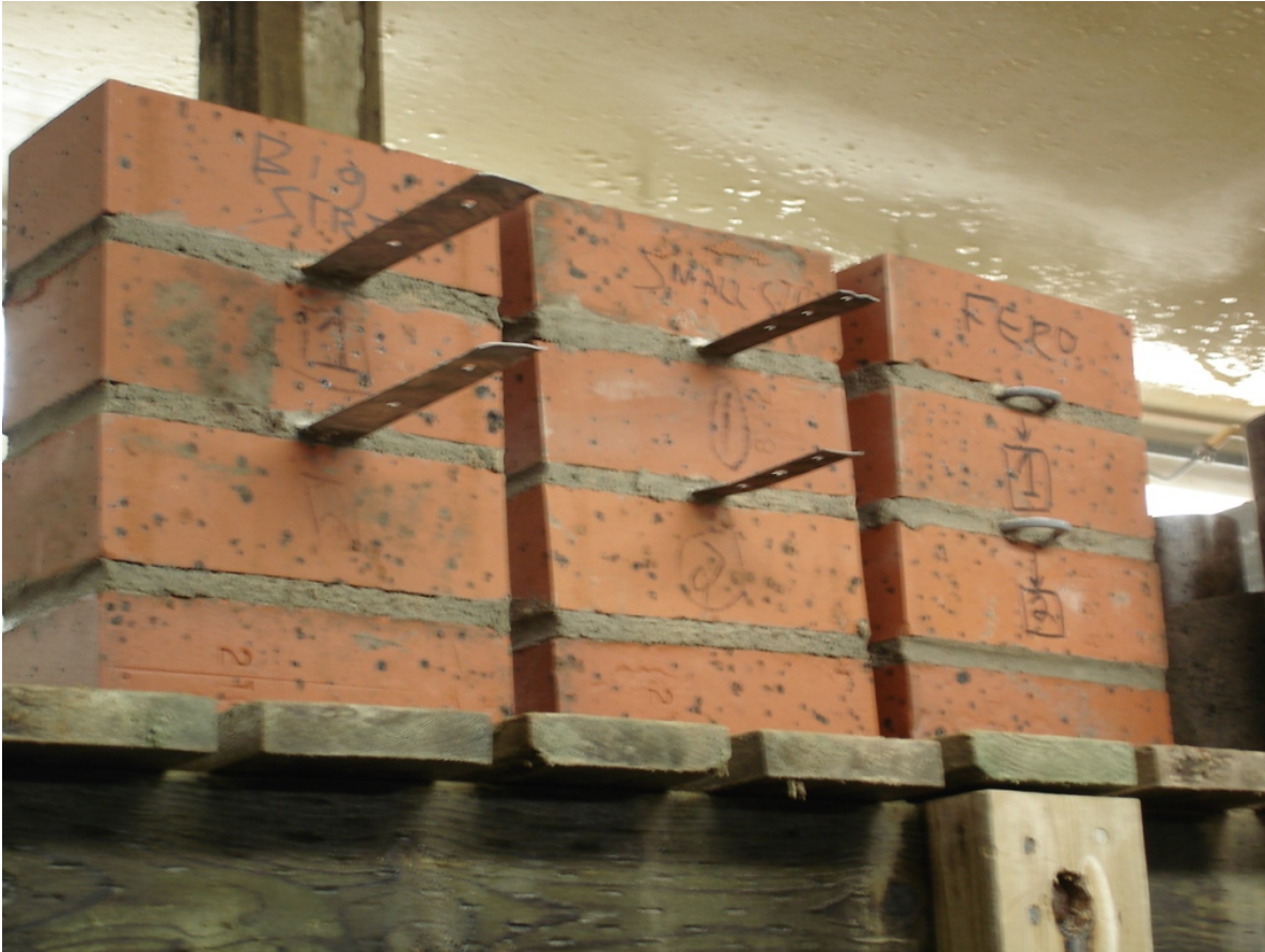
Figure 1: Brick Prisms Containing Corroding Ties
