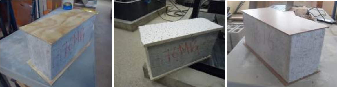
Figure 1: Illustration of the caps used in the tests, respectively: plywood, fiberboard and hardboard.
