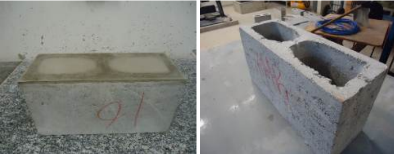
Figure 2: Blocks capped with cement paste and grinded
