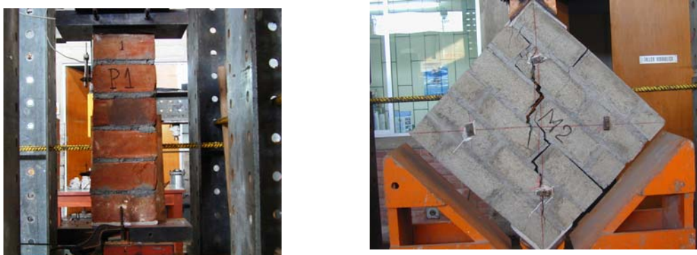
Figure 7: Tests of masonry prisms constructed by the students
