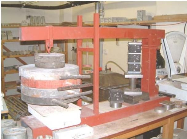
Figure 5: Creep test: a) Static deadweight load lever arm machine; b) A 50mm Demec gauge with its supporting equipment.
