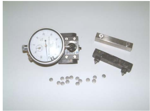
Figure 5: Creep test: a) Static deadweight load lever arm machine; b) A 50mm Demec gauge with its supporting equipment.
