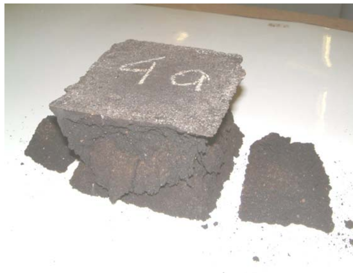
Figure 3: Brittle mode of failure of the samples.
