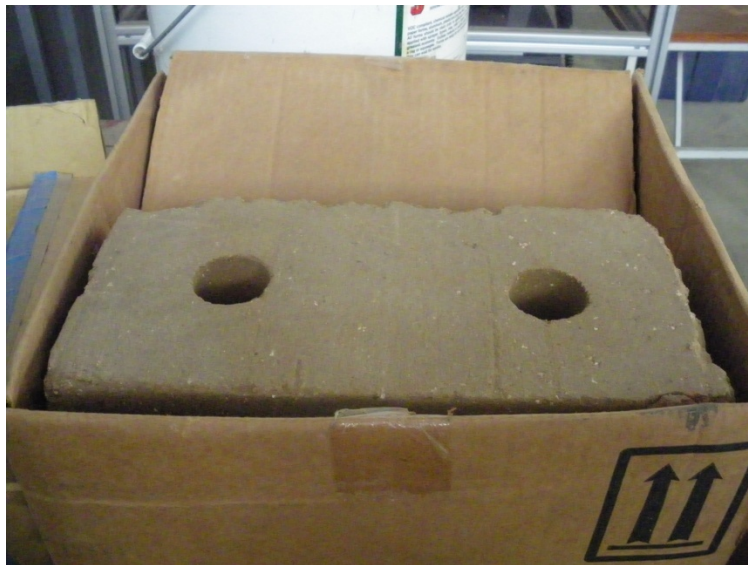
Figure 1: Moulded Earthen Block – with Core Holes for Reinforcement
