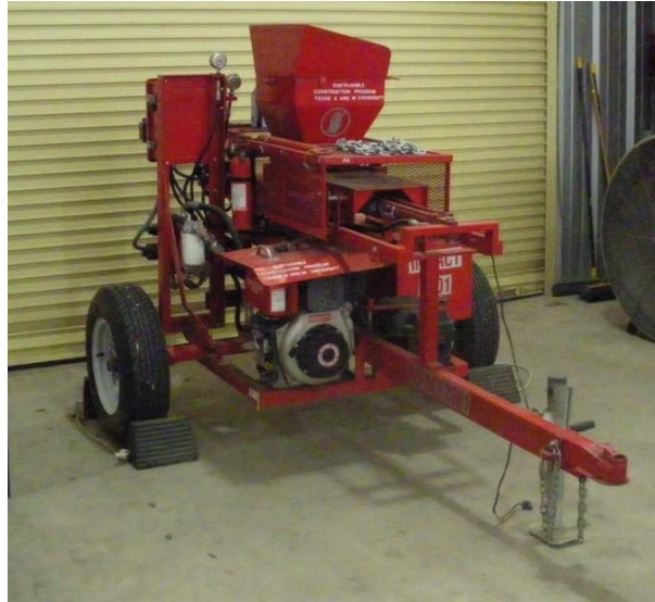
Figure 2: Moulded Earthen Block Machine at TAMU
