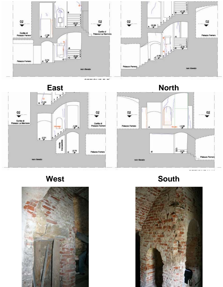
Figure 10: Crack pattern on the central pillar at ground level.
