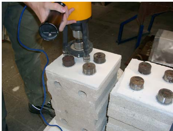
Figure 4: Test equipment for the determination of the adhesive tensile strength of the plaster according to DIN EN 1015-12 [7]
