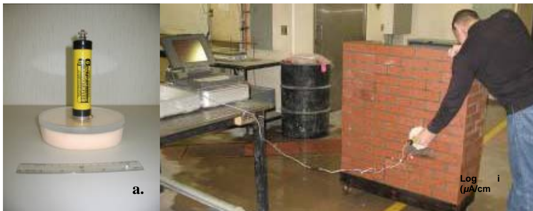
Figure 3: a) Corrosion Probe As-built; b) Apparatus/set-up use for wall specimen LPR experiments
