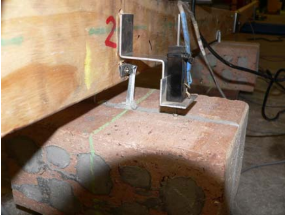
Figure 8: Tie buckling at positions 2 & 3
