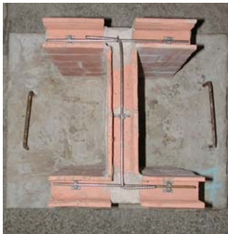
Figure 1: a) Steel bars in the bond beam; b) Steel truss; c) Steel staple
