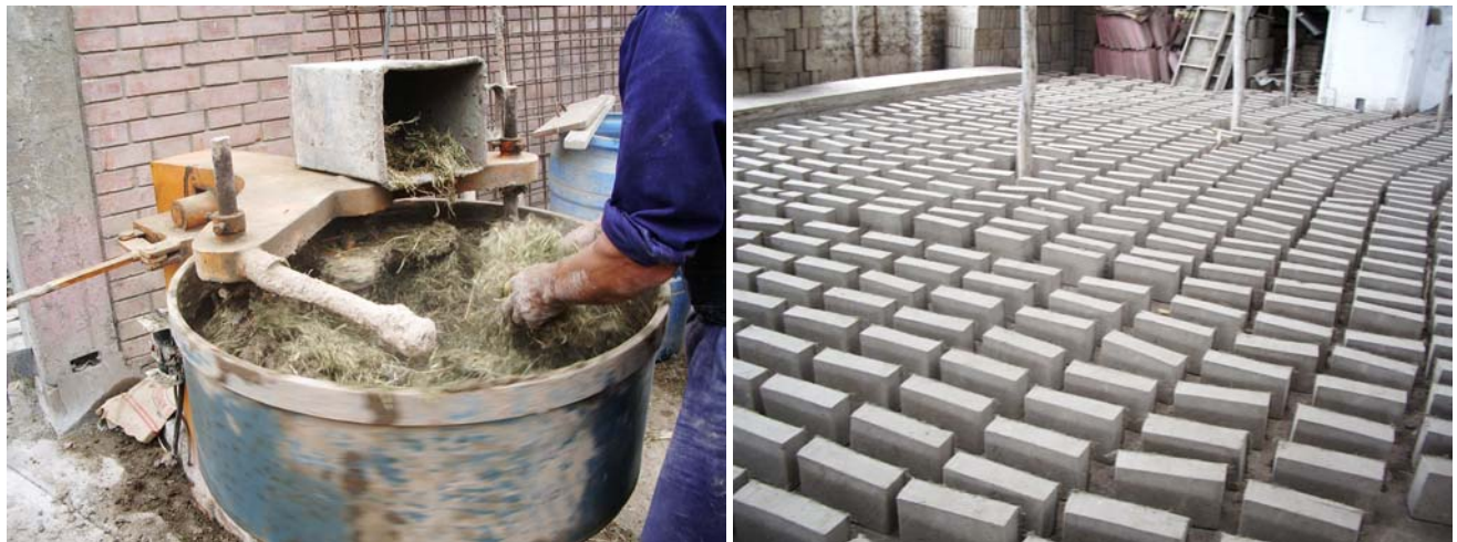
Figure 2: Preparation of adobe blocks: a) Mixing; b) Adobe blocks drying in a covered yard.
