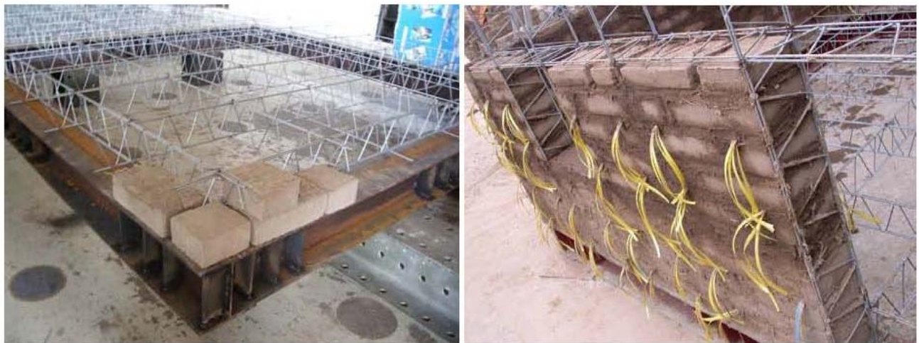
Figure 4: a) Dry test; b) Courses of adobe blockwork in the outer wall of the prototype.
