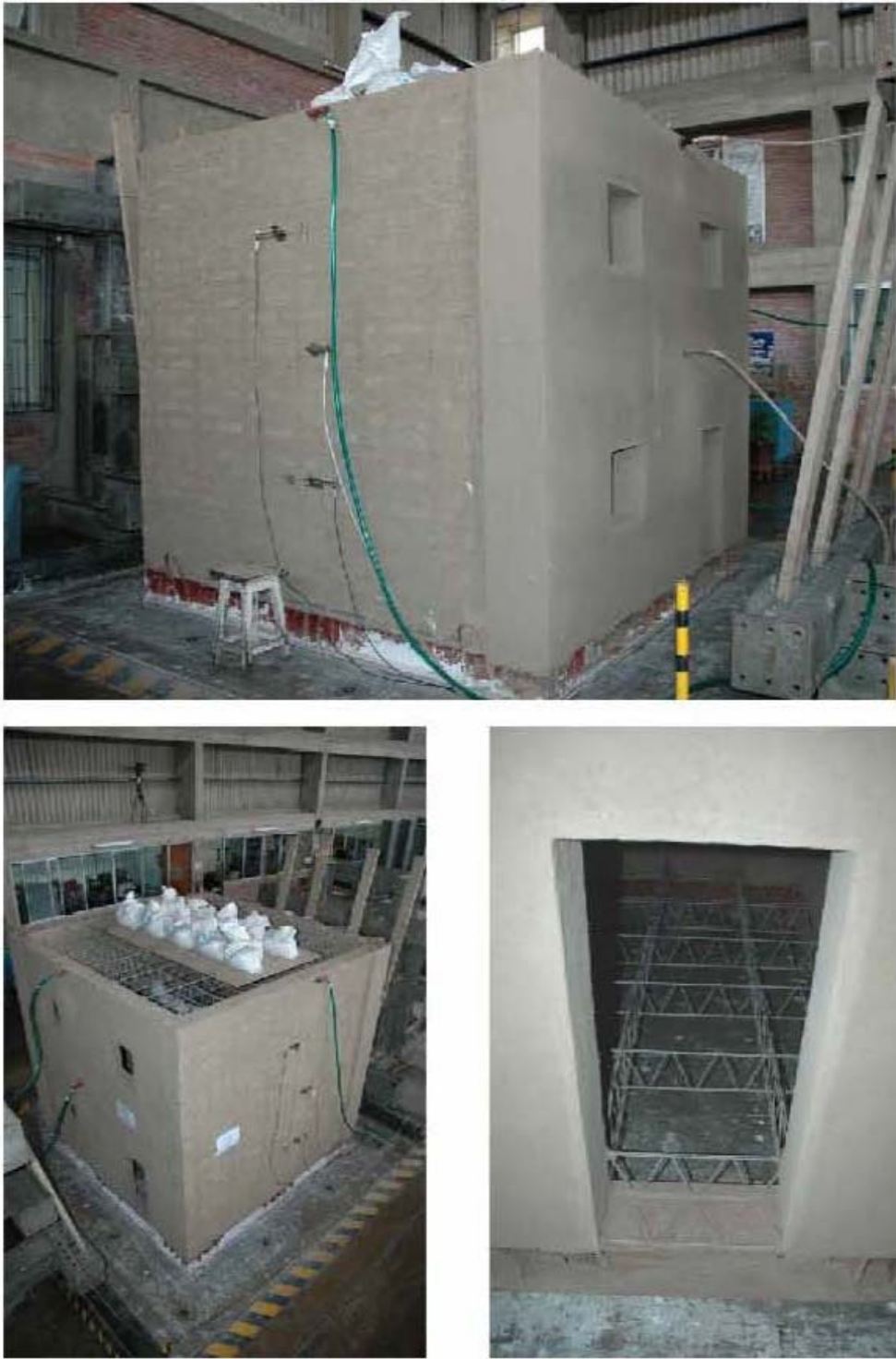
Figure 5: View of the prototype prior to earthquake resistant testing: a) On the test table; b) Upper view; c) Door.
