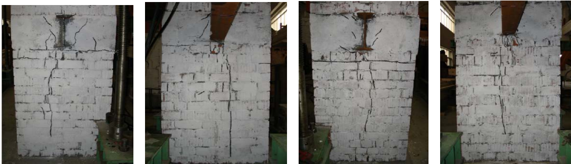
Figure 3: Failure mode of specimen
