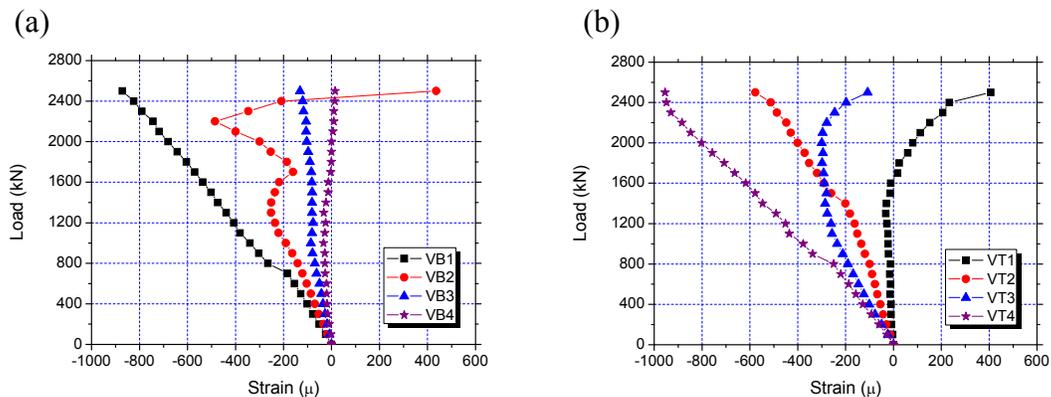
**Figure 7: Strains of vertical Bars in Masonry Wall WB2: a) In Bottom; B) In Top**
