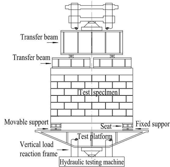
**Figure 2: Test Set-up**
