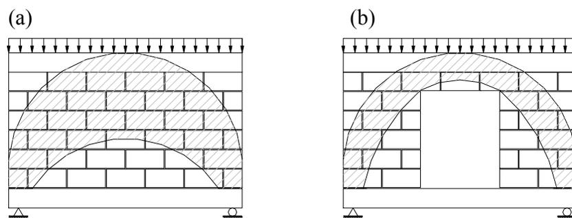
Figure 9: Arch Action of Simply Supported Reinforced Concrete Masonry Wall/Beam:
