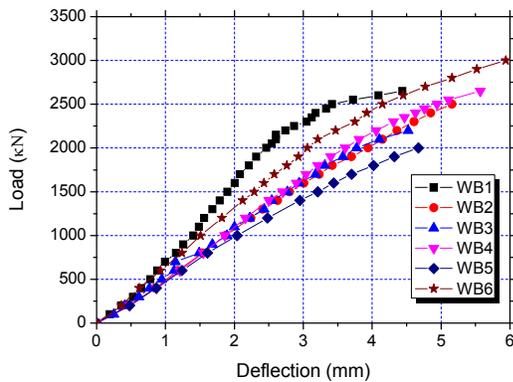
**Figure 4: Mid-Span Deflection of Specimens**
