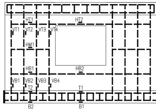
**Figure 5: Locations of Strain Gauges**
