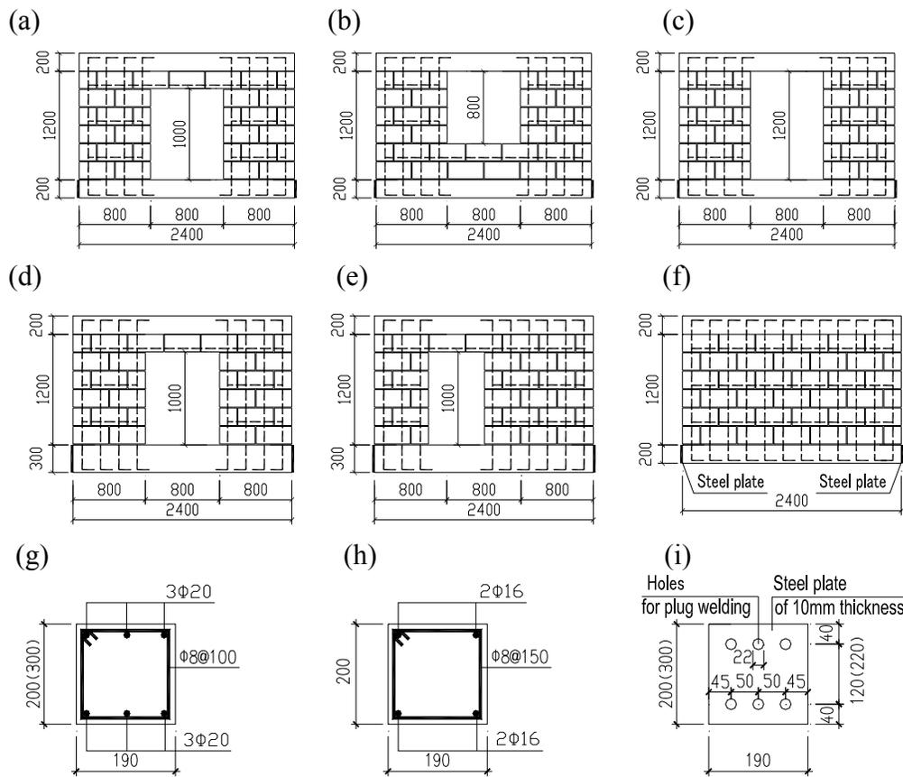
**Figure 1: Test Specimens: a) WB1; b) WB2; c) WB3; d) WB4; e) WB5; f) WB6; g) Sectional Steel for Trimmer Beam; h) Sectional Steel for Top-Beam; i) Bolting Steel Plate**
