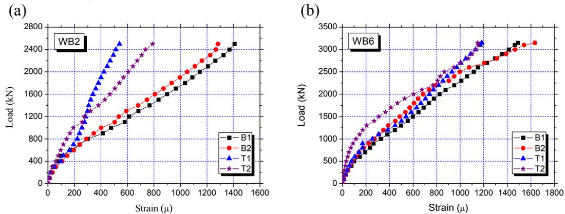
**Figure 6: Strains of Longitudinal Bars in Trimmer Beam: a) WB2; b) WB6**
