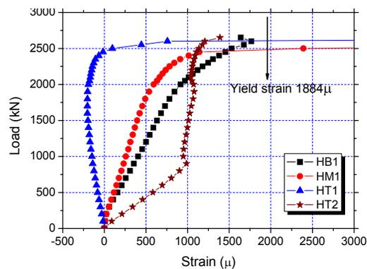
Figure 8: Strains of Horizontal Bars in Masonry Wall WB1
