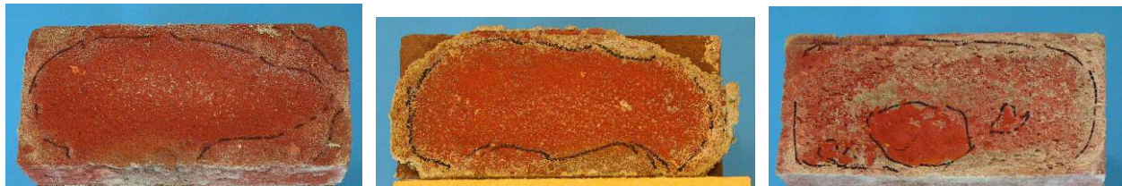
Figure 8: Irregular shaped mortar brick bond surfaces after bond wrench testing
