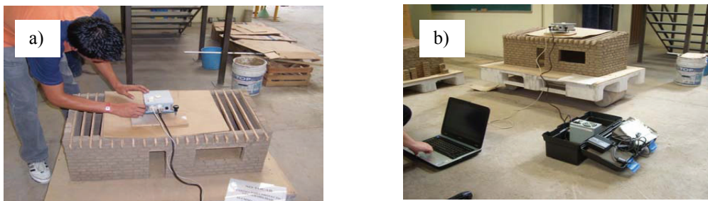
Figure 12: a) Positioning the noise tester b) Registering vibration on scale model
