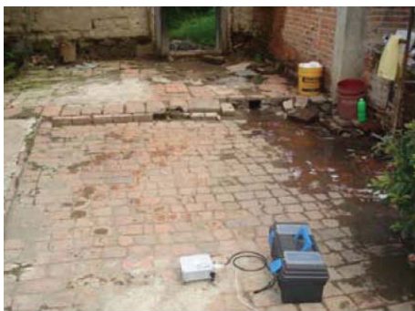
Figure 8: Registering vibration in the ground
