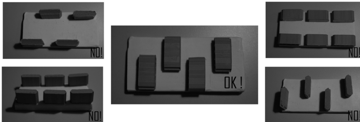
Figure 4: Correct or wrong placing of the bricks in the quarter-deck (Cristini-Ruiz Checa)
