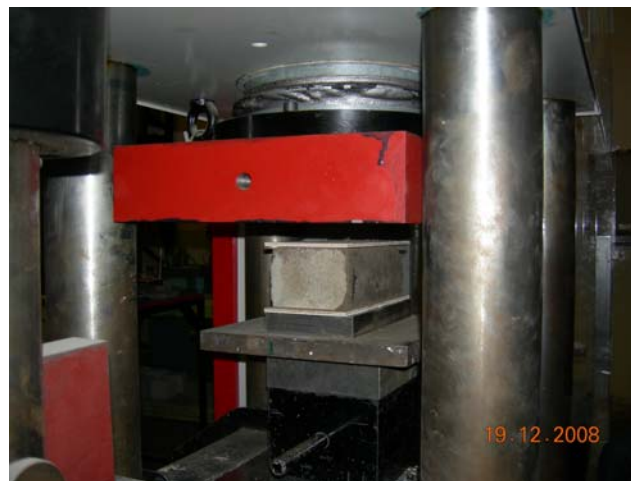
Figure 5: Configuration of the compressive strength tests.
