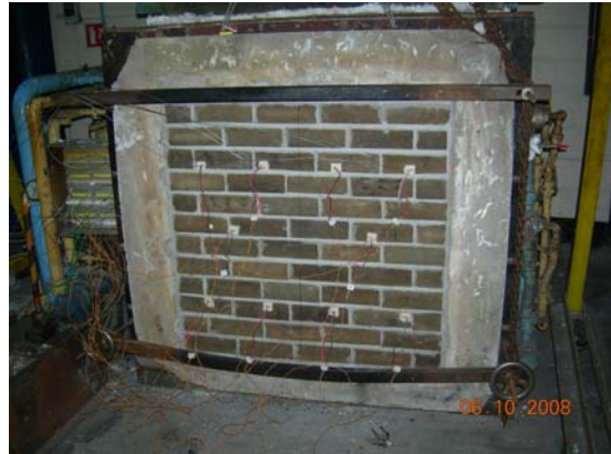
Figure 2b): The unexposed face of the test wall with thermocouples as it appeared attached to the furnace.
