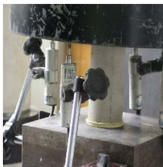
Figure 2: Additional devices for displacement measurement: a) Block; b) Mortar specimen; c) Wallet
