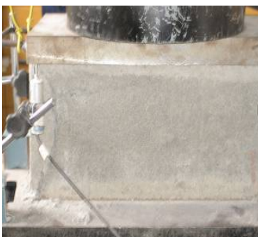
Figure 2: Additional devices for displacement measurement: a) Block; b) Mortar specimen; c) Wallet
