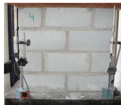
Figure 2: Additional devices for displacement measurement: a) Block; b) Mortar specimen; c) Wallet
