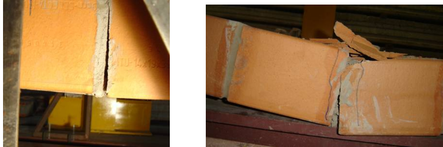
Figure 15: left) panel 1: central section during loading; right) panel 2: failure
