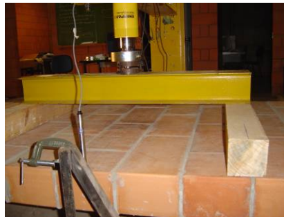
Figure 12: left) Load-cell; right) LVDT at midspan
