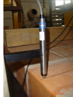
Figure 12: left) Load-cell; right) LVDT at midspan
