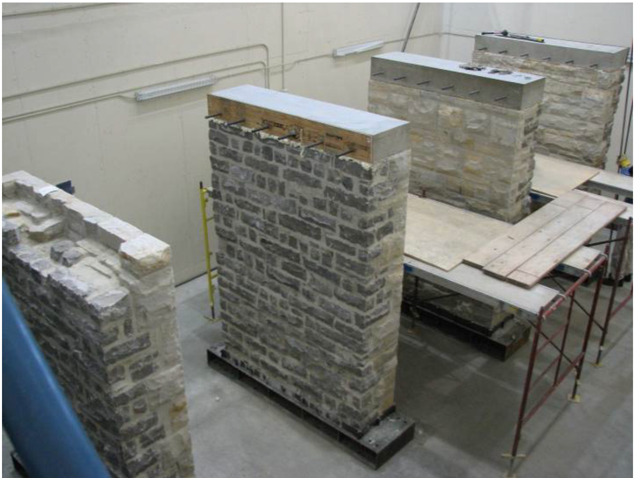
Figure 1: The walls were constructed with one side from sandstone in a sneck pattern (as seen in the two walls on the right), and the other side from limestone in a running bond pattern (as seen in the two walls to the left)
