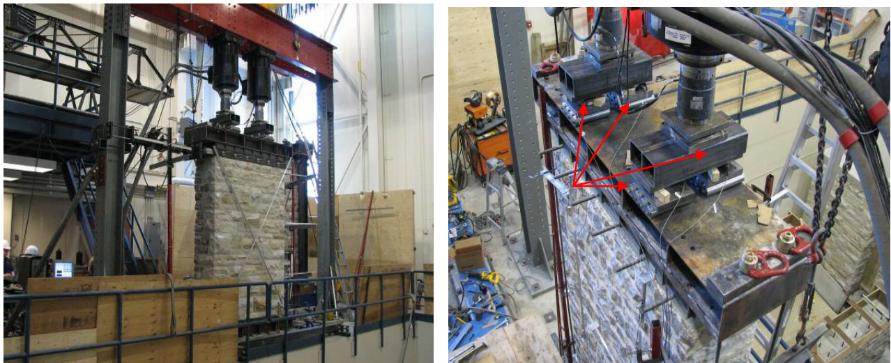
Figure 3: The testing rig (left) and the four loading points shown with arrows (right).
