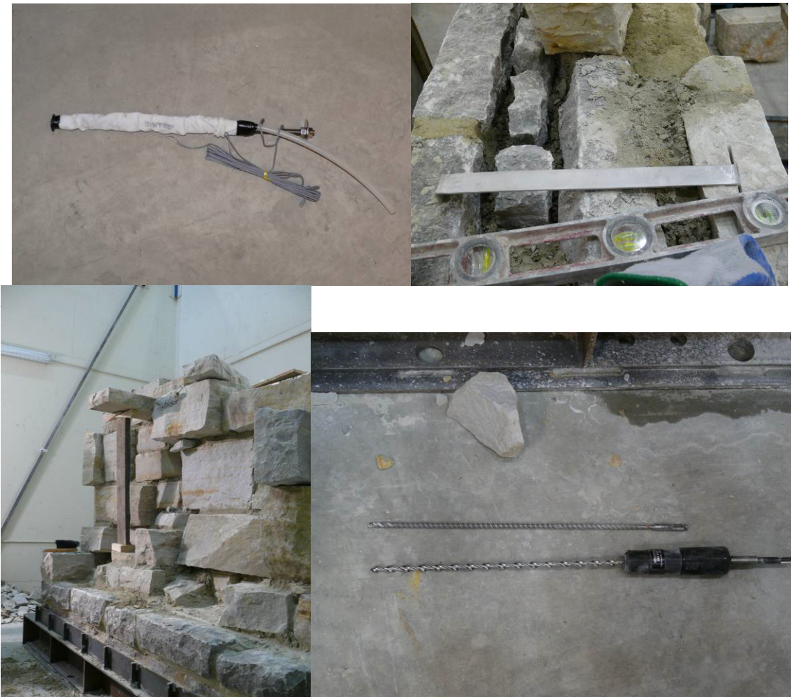
Figure 2: Examples of the different anchoring types: top left Cintec anchor, top right Stainless Steel Cramps, bottom left overlapping stones, and bottom right Helifix anchors
