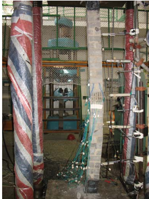
Figure 6: Photo of Lateral Bending of Column (ZM-5)
