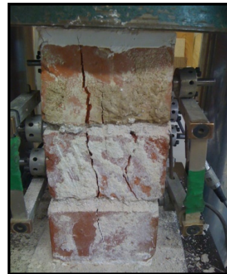
Figure 5: Cracks developed during prism test
