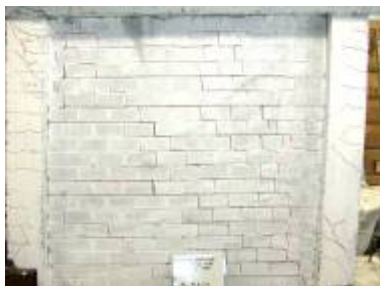
d) Maximum deformation reached at Drift 3.55%
