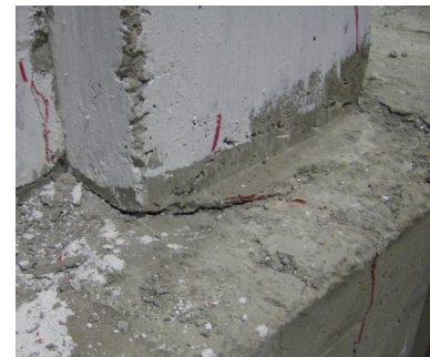
f) Compression column Drift 3.55%
