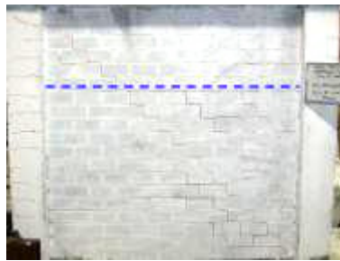
b) Shear Sliding at Drift 1.00%
