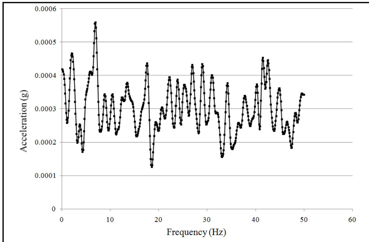
**Figure 7: Building One – Out of plane – FFT of Acceleration Z**
