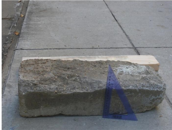
**Figure 5: Test Building – Measurement at Mounting Point C – 150 mm Kerb Point**
