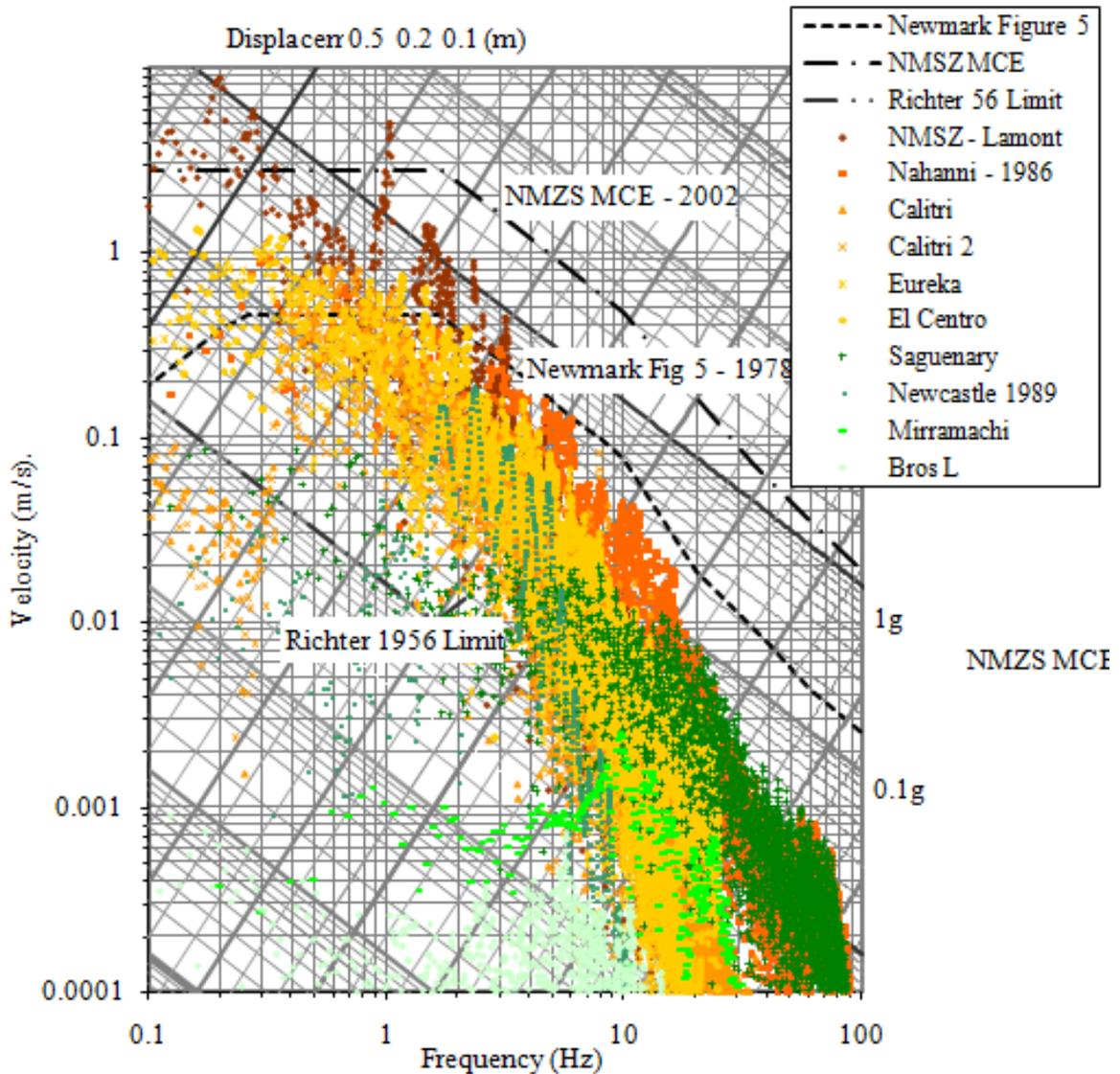
**Figure 2: Seismic Standard Evolution 1956 - 2003**
