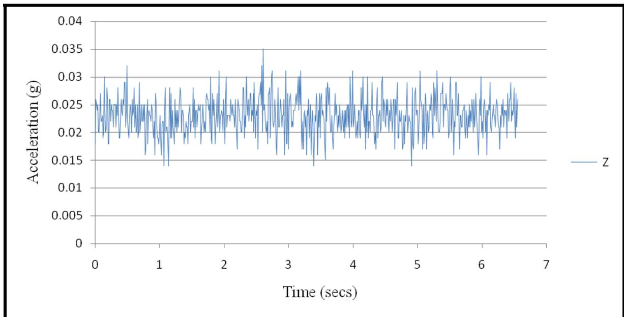
**Figure 6: Building One – Out of plane - Acceleration on Wall – Loading F150 Ford**
