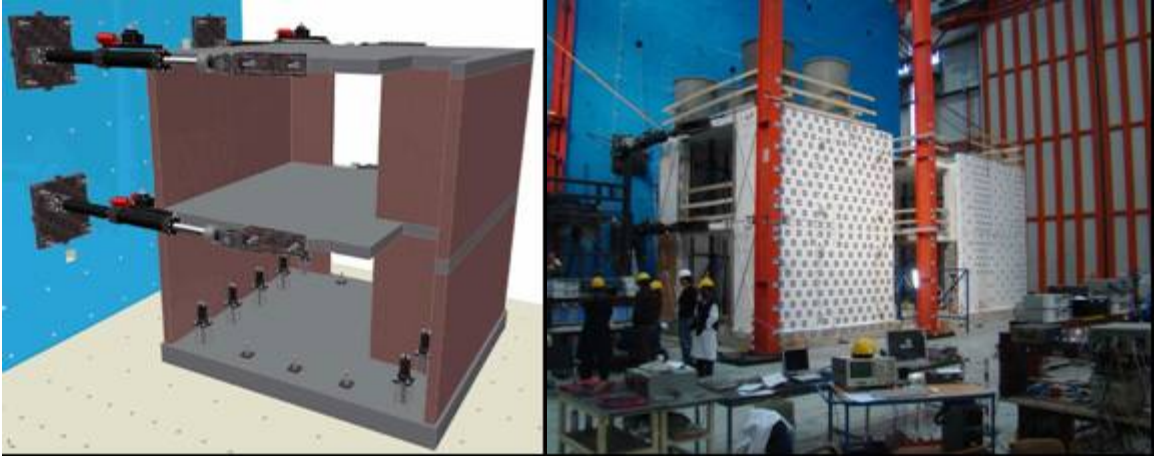
Figure 5: Specimen for the pseudo-dynamic tests; schematic diagram (left) and “ready for testing” (right)
