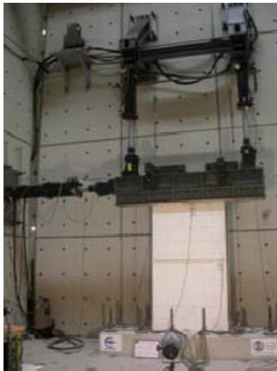
Figure 2: Test set-up for static-cyclic in-plane shear tests in Pavia [9]
