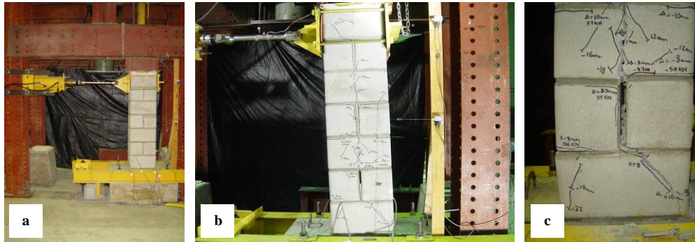
Figure 5: (a) Control specimen before test (b) Column at 2% drift level (c, d) Sample of cracks and spalling at column's base (e) Column at 5% drift level
