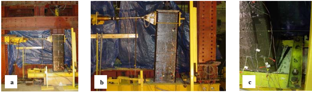
Figure 7: (a) Wrapped column before the test (b) Specimen at 5% drift level (c) Wrap rupture near the base
