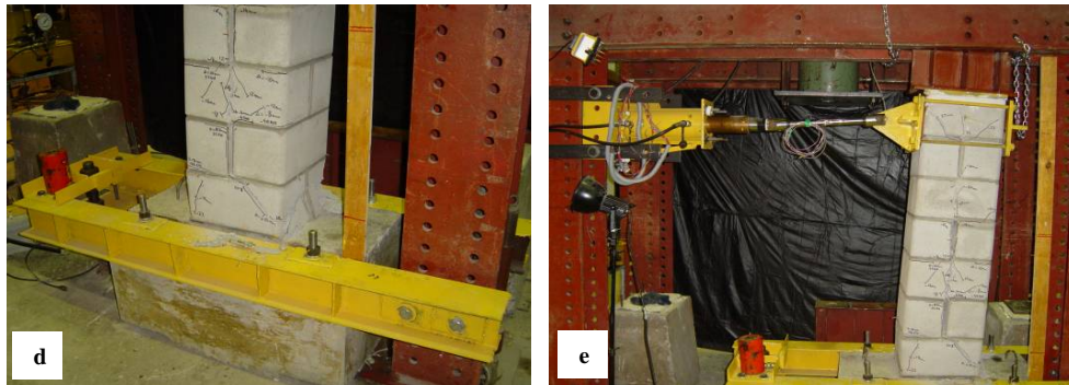
Figure 5: (a) Control specimen before test (b) Column at 2% drift level (c, d) Sample of cracks and spalling at column's base (e) Column at 5% drift level
