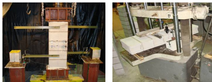
Figure 1: Tests for obtaining compressive (left) and tensile (right) strength of masonry assemblage
