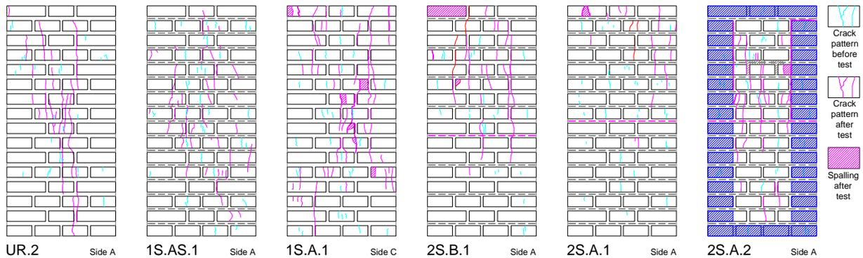
**Figure 4: Crack patterns of some strengthened masonry panels after standard compression test. Only for specimen “2S.A.2 - Side A” inclined hatch on the perimeter represents external CFRP sheets.**
