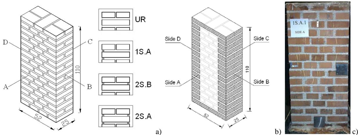
**Figure 2: a) Masonry panels dimensions and reinforcement configurations; b) application of CFRP sheets around corners, c) specimen 1S.A.1 after compression test.**
