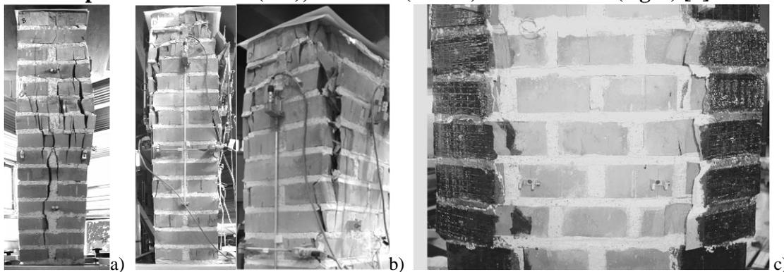
**Figure 9: a) Crack pattern of the specimen UR.3.C, b) crack pattern of 2S.A.3.C with material spalling, c) crack pattern of 2S.A.4.C with peeling of CFRP sheet [5].**
