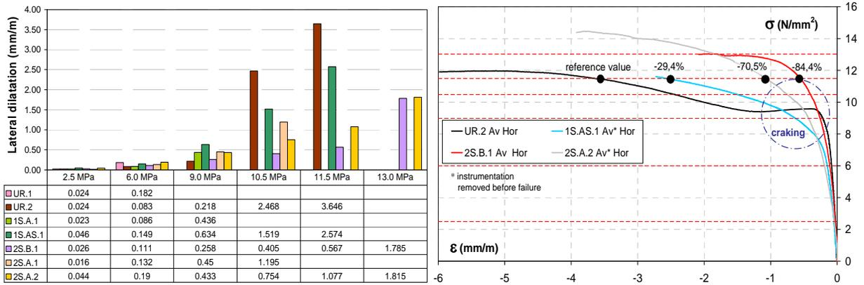
**Figure 3: (left) Comparison of lateral dilatation of the strengthened specimens at different compressive levels; (right) lateral dilatation of some specimens with percentage variation at the compressive stress of 11.5 N/mm<sup>2</sup>.**
