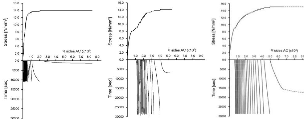
**Figure 8: Compressive stress and time vs. horizontal deformation of sides A and C of the specimens UR.3.C (left), 2S.A.3.C (centre) and 2S.A.4.C (right) [5].**
