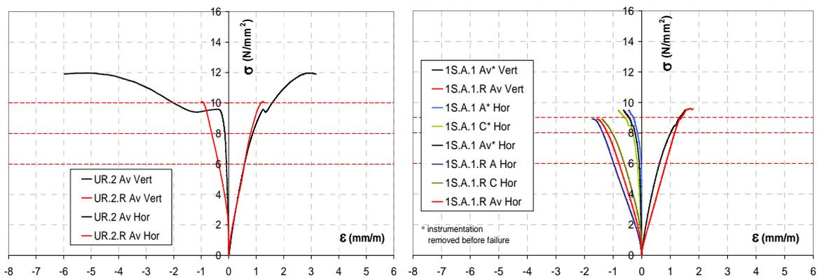
**Figure 5: Comparison of lateral dilatation of the repaired specimens, (left) UR.2 versus UR.2.R and (right) 1S.A.1 versus 1S.A.1.R.**
