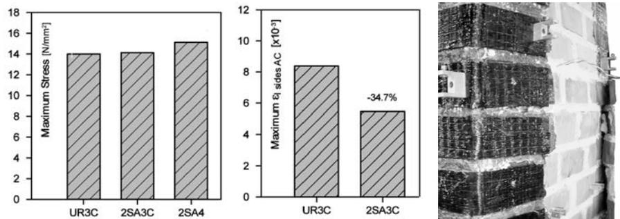
**Figure 7: Maximum compressive stresses (left), and maximum horizontal deformations measured in the accelerated creep tests (centre). Test 2S.A.4.C: the CFRP sheet detachment interferes with horizontal transducers (right) [5].**
