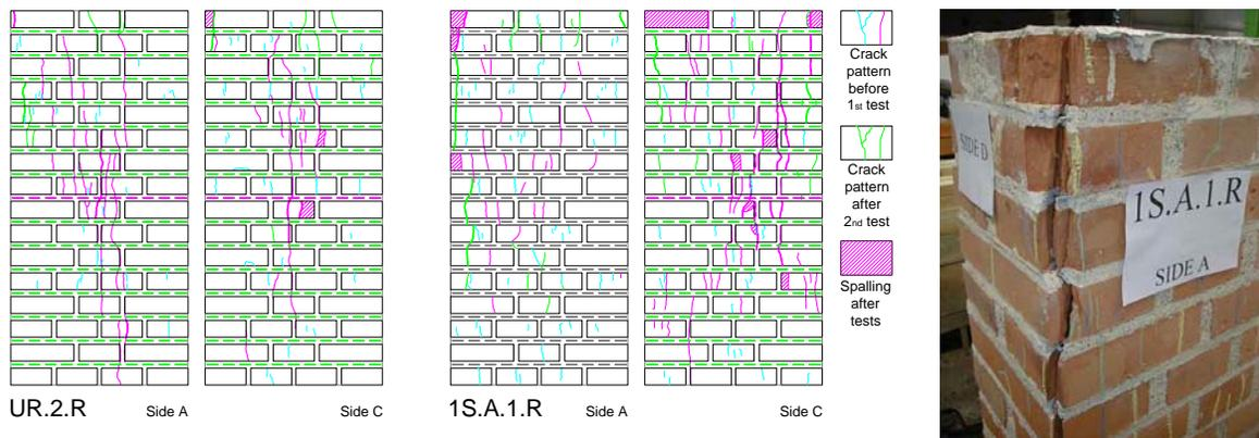
**Figure 6: Crack patterns after test of repaired panels (left), and corner detail (right).**
