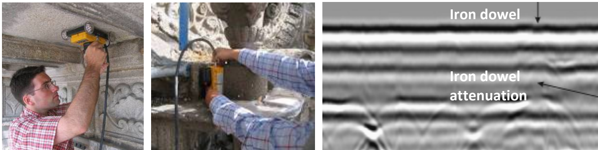
Figure 27: Aspects of the GPR Inspection.
