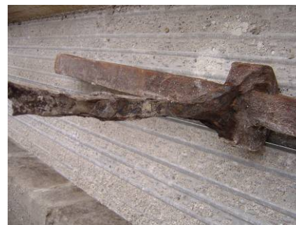
Figure 9: Ancient Tower Ties: (a) Deformed Anchorage ( T_1 ); (b) Details of Broken Tie ( T_3 ).
