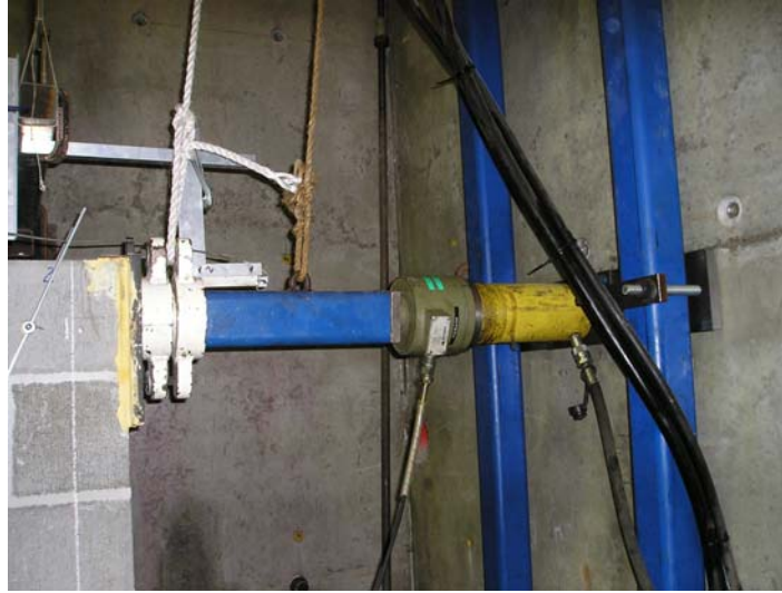
Figure 5: The actuator for applying lateral in-plane load at the top of one end of the wall.
