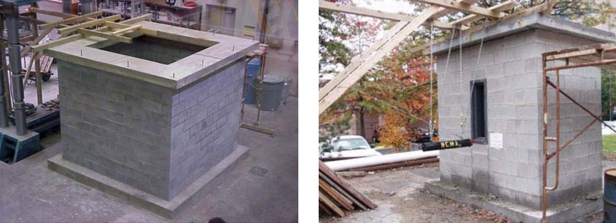
**Figure 3 – Prison Impact Test Walls**
