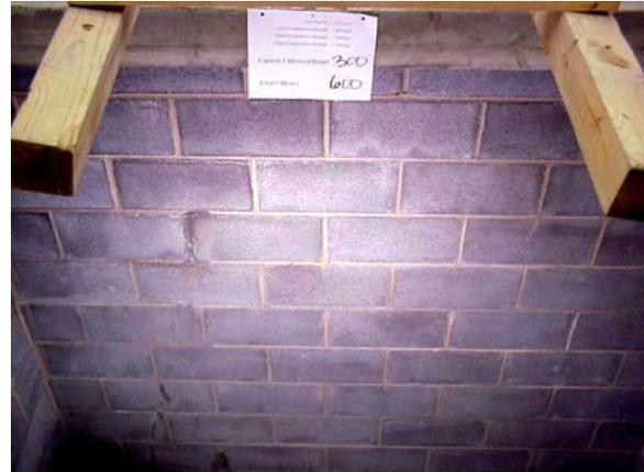
**Figure 7 – Typical Wall Condition After 600 Blows – Rear Side**
