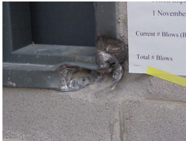
**Figure 9- Close-up of Window Frame Damage at 935 Blows**
