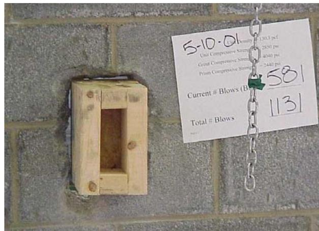
**Figure 8 - Typical Breach Failure**
