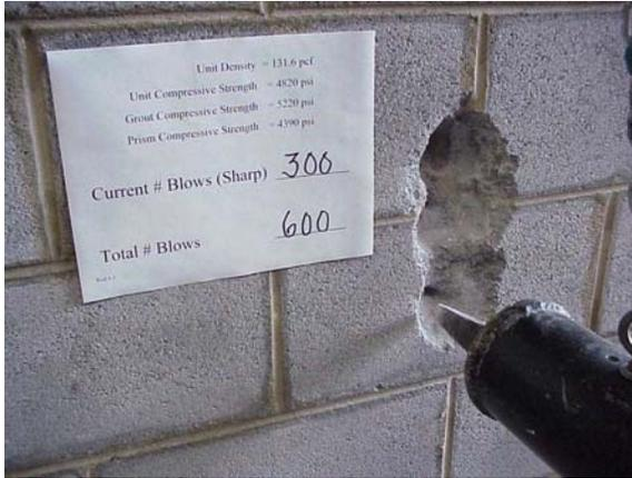
**Figure 6 – Typical Wall Condition After 600 Blows – Front Side**
