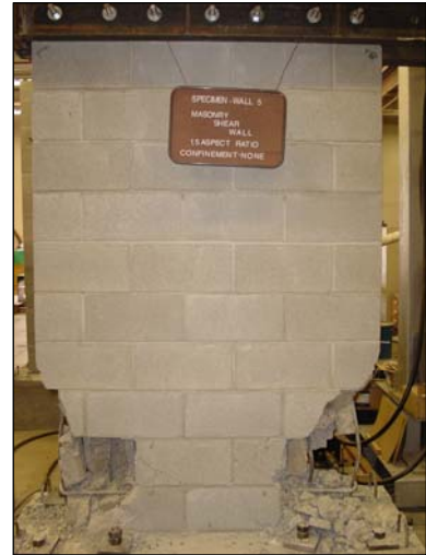
Figure 4 - Wall 5 After Testing
