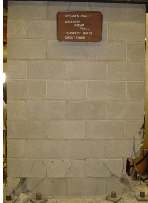
Figure 10 - Wall 8 After Testing
