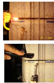
b) Horizontal cracking in Wall 1
