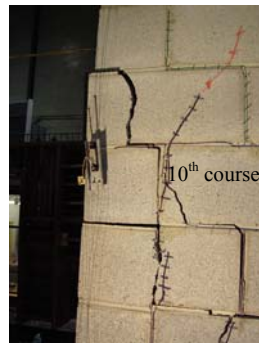
a) Vertical cracking at East end of Wall 1
